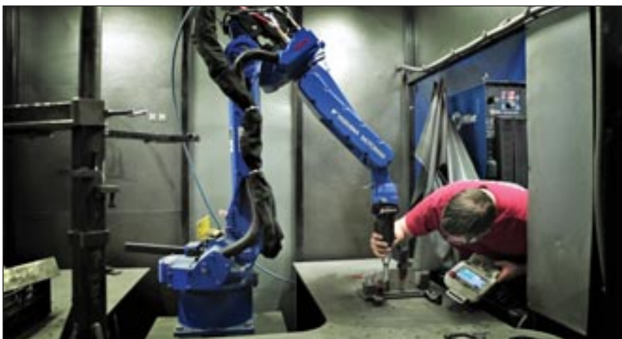
Using Kinetiq Teaching™, a technician hand-guides the robot arm to a weld point, thereby teaching the robot its job.
