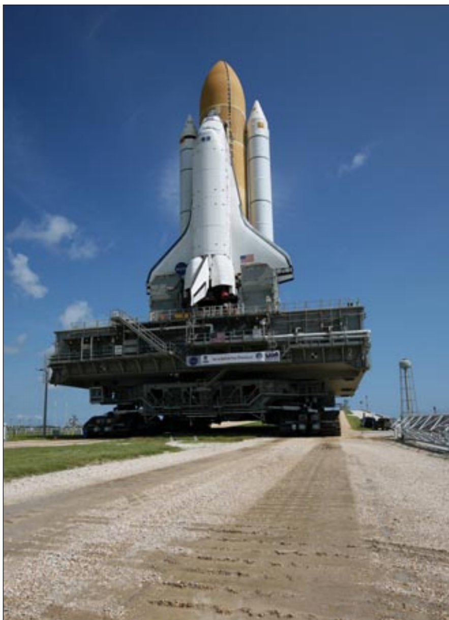
When they were built, Kennedy Space Center's crawlers were the largest tracked vehicles ever made. The two crawlers were used for transporting the space shuttles.
