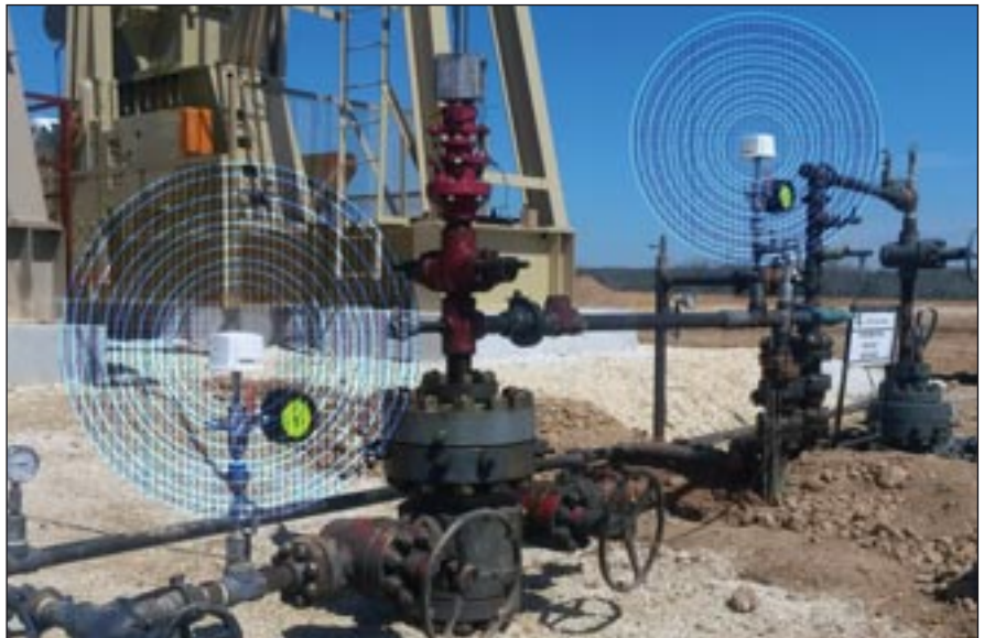
Figure 3. SignalFire Wireless Telemetry, a Hudson, MA-based company that offers remote asset monitoring and control services, now implements the Advanced Encryption Standard (AES) with a 128-bit key size to protect its wireless data. A SignalFire wireless node is shown in the above image.
