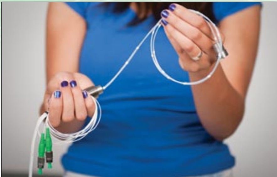
The CryoFOSS system includes a fiber optic connector and sensor. (Image Credit: NASA)
