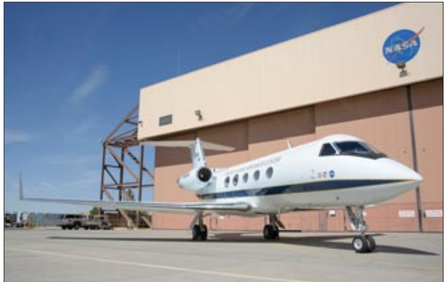
The modified Gulfstream III (shown) is the testbed aircraft for the ACTE flexible-flap research project. (Image Credit: NASA)
