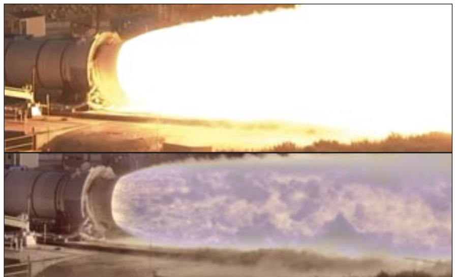
(Top) Image of the Space Launch System test without using the HiDyRS-X camera, and (bottom) with the HiDyRS-X camera.
