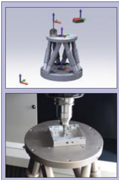
PI hexapods can work with multiple coordinate systems and allow the user to change the center of rotation or cast/rotate a coordinate system with a simple software command — an important feature when using the hexapod in precision machining applications. (PI)
