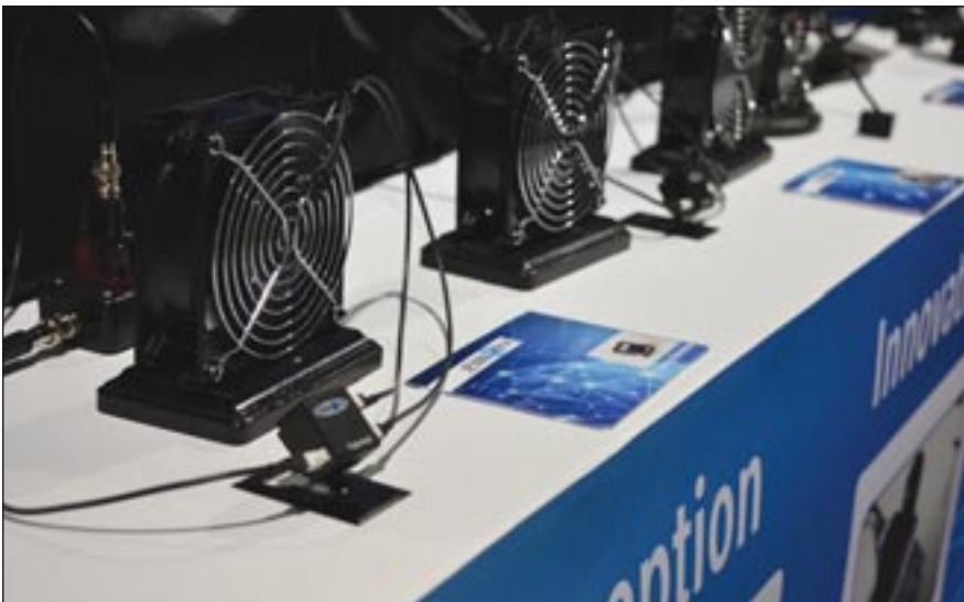
An expo display of rotation-based energy harvesters, gathering energy from standard fans. In this example, up to 18 mW is possible from a single energy harvester. (Image Credit: Jennova)
