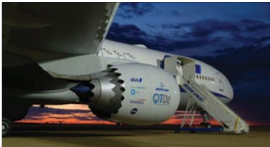
Chevron flow effectors are part of this engine nozzle chevron design that uses asymmetrical scallops around the engine to reduce noise. (Credit: The Boeing Company/Bob Ferguson)
