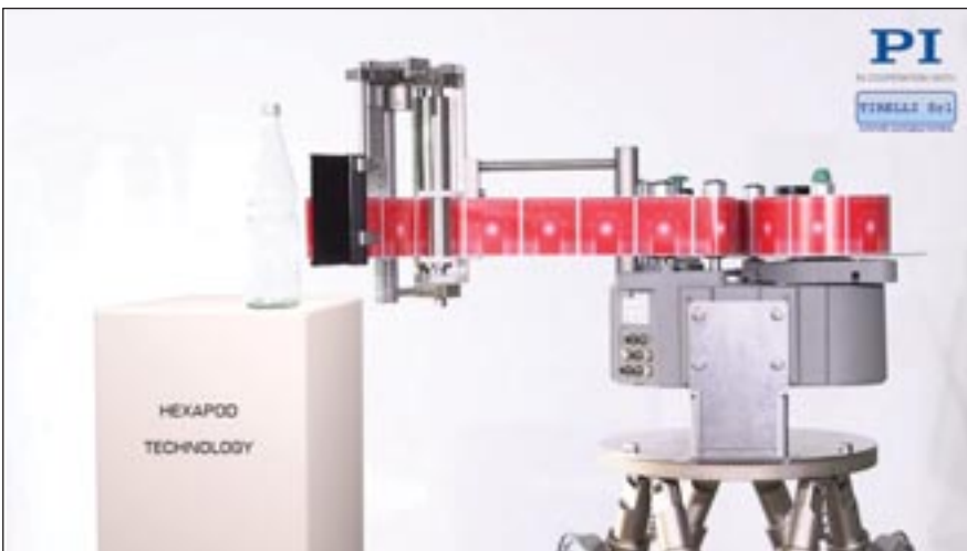
Hexapod in a labeling robot prototype. (Tirelli/PI)
