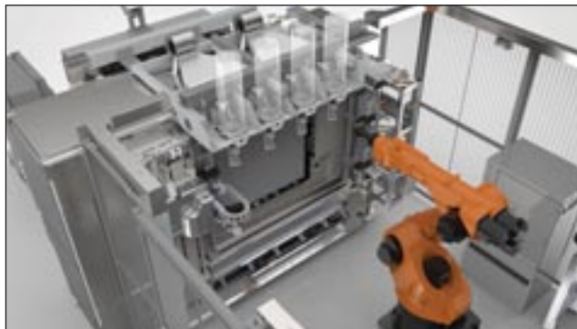
The Infinite-Build 3D Demonstrator produces large tools and production parts with part-to-part repeatability.
