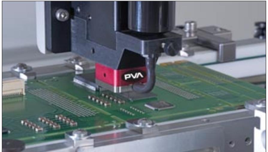
A JDX valve used in underfill of sensitive electronic components. (Credit: Precision Valve & Automation)
