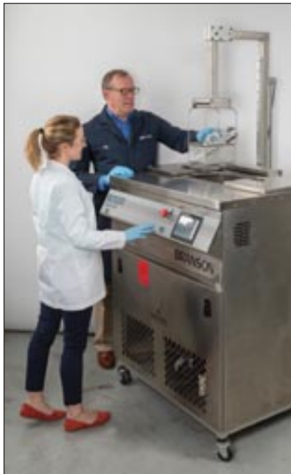
Jay Tourigny, MicroCare senior vice president and Venesia Hurtubise, a chemist with the company, develop a cleaning protocol for a large metal casting in a Branson vapor degreaser. There are numerous factors that can be tweaked in vapor degreasing to optimize cleaning results, throughput, or costs, depending on the goals of the organization.
