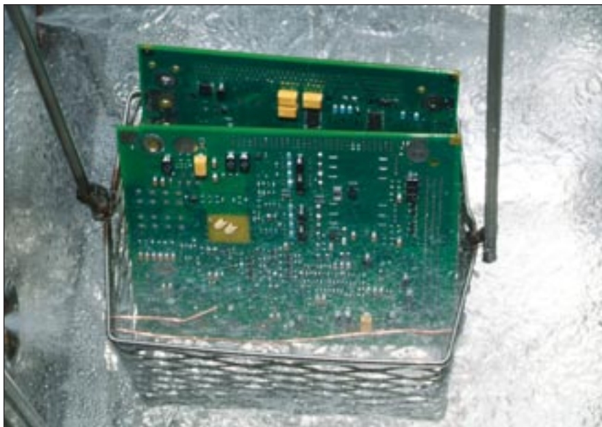
Modern electronics are easily cleaned in a vapor degreaser because the solvent can be tailored to precisely match the contamination. Importantly — and unlike aqueous cleaners — vapor degreasing is highly scalable, so a small benchtop machine cleans exactly as well as a large, floor-mounted system.
