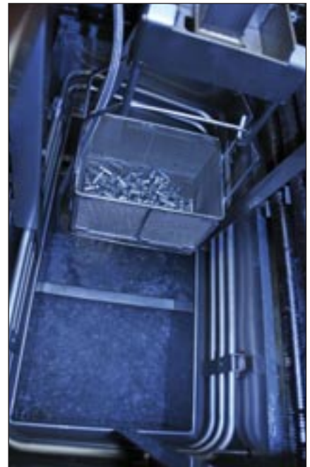
Vapor degreasers excel at cleaning optical devices, ceramics, PCBs, or metal pieces like these fuel injectors. Solvent cleaning systems are well suited for parts with small apertures, tight stand-offs, and blind vias. Because solvents offer substantially better wetting than aqueous cleaners, they are the optimal choice on complicated shapes, small parts, fragile devices, or in high-volume cleaning environments.
