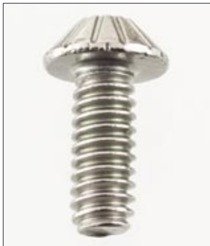
This net shape micro-screw produces no scrap and has an increased tensile strength due to work hardening through the cold forming process.
