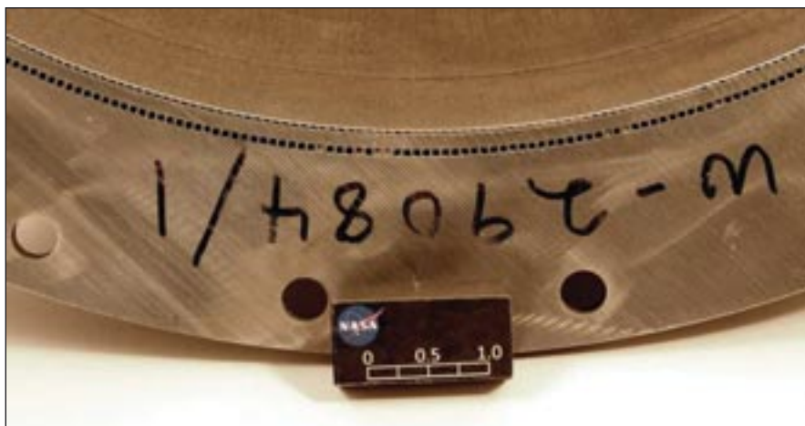
Interim inspection improves the quality of parts with intricate internal features like these fuel channels.
