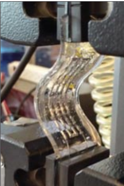
Liquid metal in the flexible thermoelectric device allows for self-healing — rigid devices do not have this ability. (Mehmet Ozturk, NC State University)
