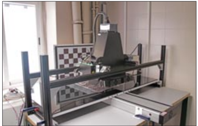
Figure 3. Chromasens truePIXA camera systems permit color measurement on two-dimensional objects, especially for print inspection.
