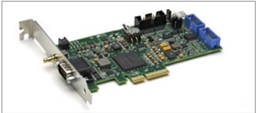
Figure 1. The Aon-CXP single-link CoaXPress frame grabber designed for use with low-cost, compact CXP single-link cameras.
