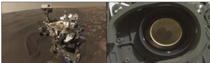
(Left) NASA’s Curiosity rover uses an XRD device called CheMin to analyze minerals in the Martian soil. The key innovation of CheMin was that it didn’t require samples to be finely ground into powder; in fact, the rock grains need only to be small enough to fit through the screen installed on Curiosity (right), through which the rover funnels the samples it collects with its robotic arms.
