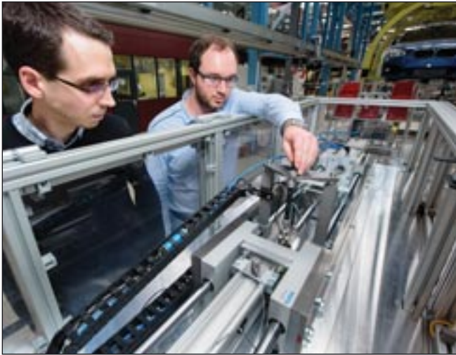
Researchers test the smart condition monitoring system on an electro-mechanical cylinder. (Oliver Dietze)
