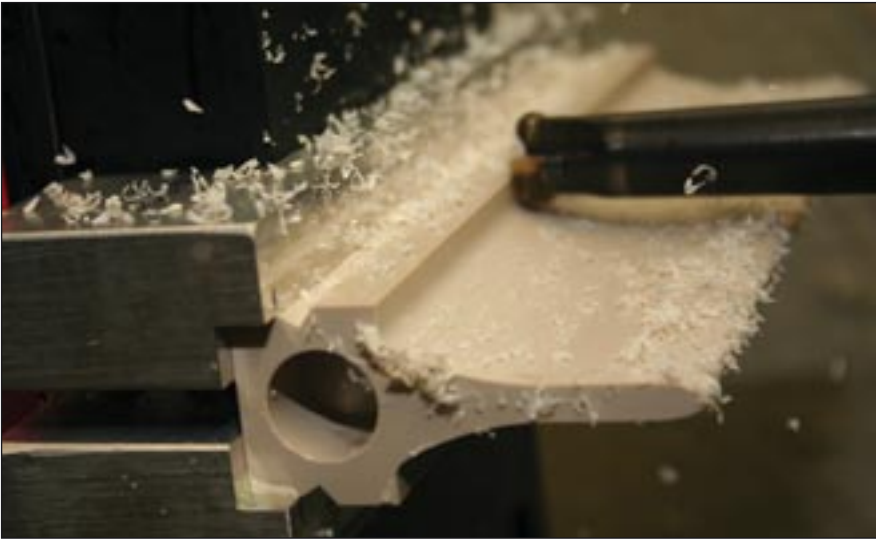
Thermoplastics can be machined to extremely tight tolerances up to 0.002mm, which can be critical for aerospace.
