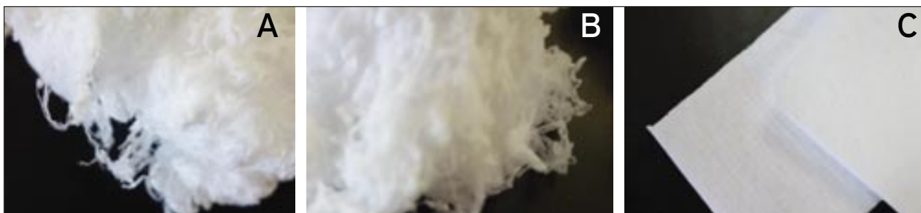
Images of as received nanofiber materials: hydrophilic (A), hydrophobic (B), and sheet type (C) variations.
