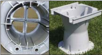
Cross sections of gas assist parts.
