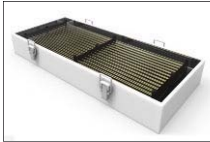
The technology is based on local redistribution of a magnetic field with the help of a metasurface made of metal resonators. [Credit: ITMO]
