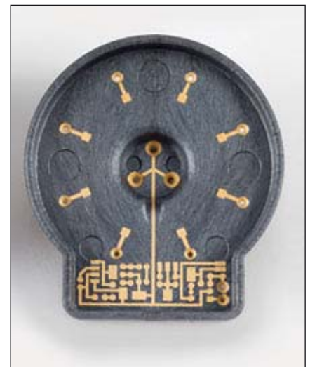
Fig. 2 - There are eight antennas surrounding the emitter on the front of the MID.
