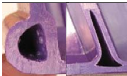
These two images show cross sections of parts created with gas assist molding.
