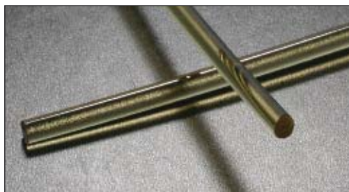
PEI, commonly known by the brand name Ultem, is the highest strength polymer of the amorphous materials.
