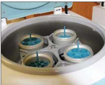
Refrigerated centrifuge (-20° to 40 °C), for PCR, DNA, and RNA, and analysis.
