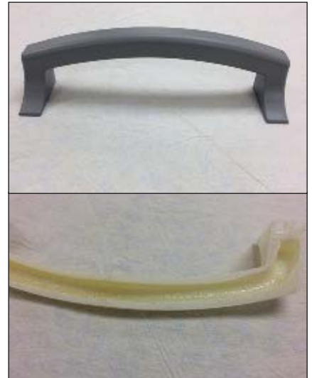
Gas assist molded handle and cross section.
