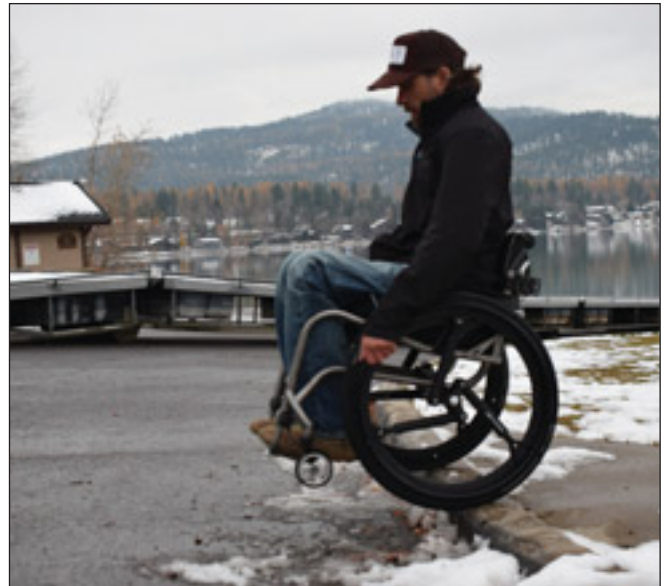
SoftWheels enable wheelchairs to roll off curbs with ease.
