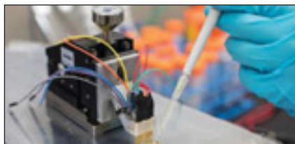
The sensor can measure the amount of critical metabolites, such as lactate or glucose, that are present in sweat, tears, saliva, or blood, and, when incorporated into a diagnostic device, could allow health conditions to be monitored quickly, cheaply, and accurately. (Credit: University of Cambridge)
