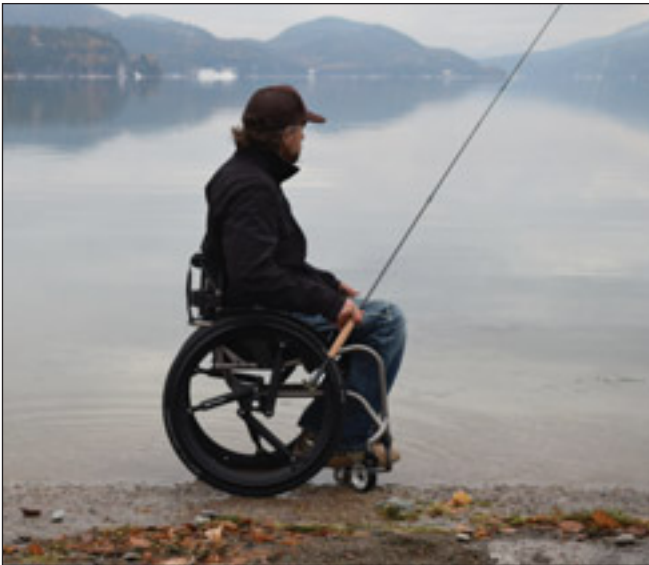
The technology acts as shock absorbers when the wheelchair encounters an obstacle or rough terrain.
