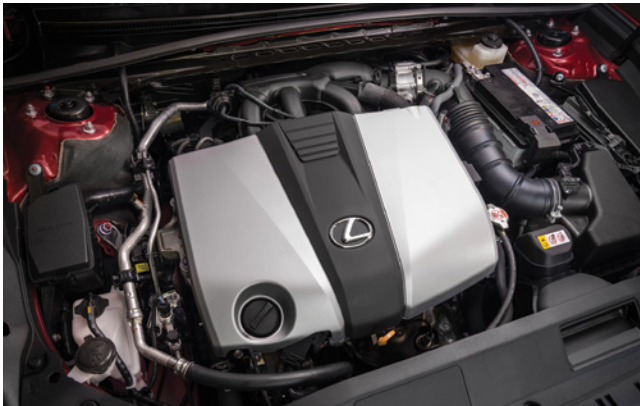
For the 2019 ES350, the 3.5-L V6 is enhanced with the D4S fueling system, which helps to extract an additional 34 horsepower.
