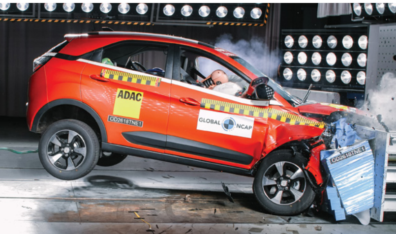
The moment of truth during the 2018 Global NCAP crash test of Tata Motors' new Nexon. The compact SUV achieved a four-star adult occupant rating and a three-star child occupant rating.
