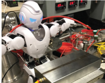
This robot quickly and efficiently detects leaks in a lithium-ion battery.
