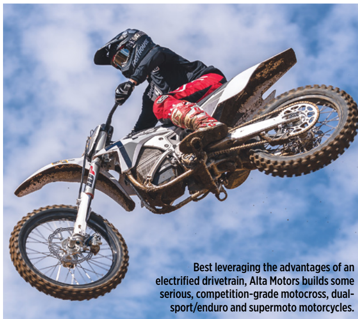
The Alta forged aluminum mono-shock chassis serves as the backbone of each of the manufacturer's five models.
