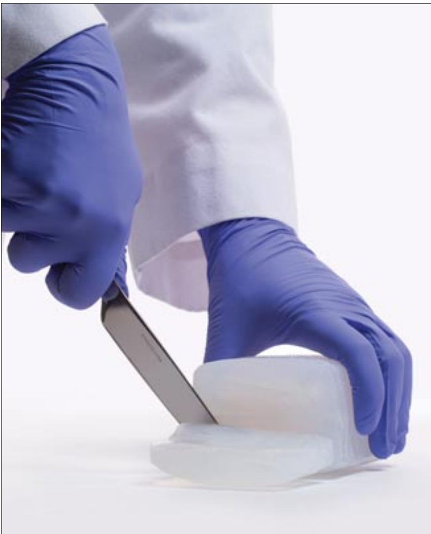
High-consistency rubber (HCR) consists of a high molecular weight polymer combined with silica to produce a material that can be molded, extruded, or calendared into a useful component. (Credit: NuSil)
