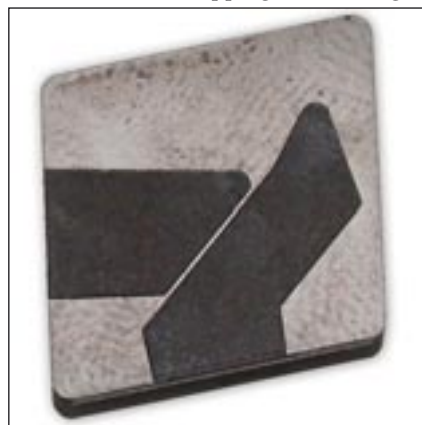
The low-cost tooling insert embedded with smart sensors. (Credit: AMRC)
