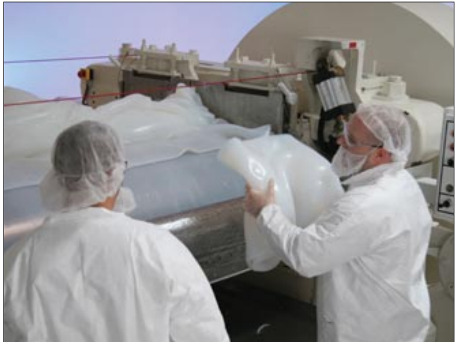
Two-roll mill processing. (Credit: NuSil)
