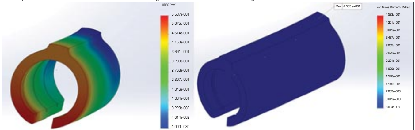
The device is a composite support with a soft polymer shell and a thin aluminum, steel, or carbon fiber sheet running the length of the apparatus to provide rigidity. (Credit: Kennesaw State University)
