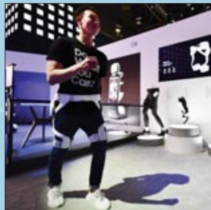
Short for Gait Enhancing and Motivating System, Samsung's GEMS assists users with walking and can also help them strengthen their muscles and improve their mobility and balance. (Credit: Samsung)
