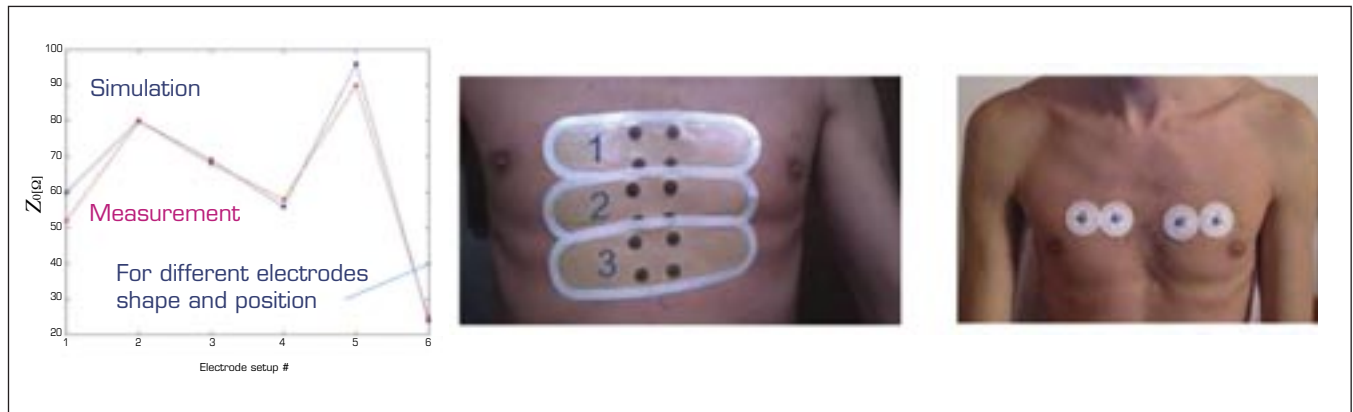
Fig. 5 – Comparison between measured and simulated bioimpedance values (left) for different electrode shapes and positions (right).
