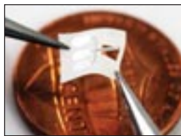
An implantable sensor has the speed and precision for tracking a brain chemical known to be elevated in certain brain diseases and after a spinal cord injury. (Credit: Purdue University image/ Tran Nguyen)
