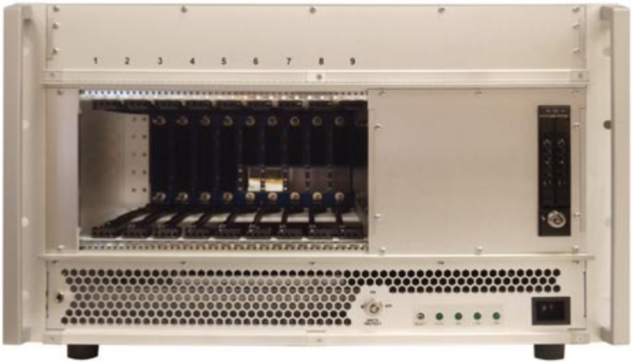
Figure 1. Commercial-grade OpenVPX chassis are commonly used for benign-environment defense applications and for prototyping. With powerful reverse-impeller blowers directly above the card guide, there is efficient cooling for even the hottest OpenVPX cards.
