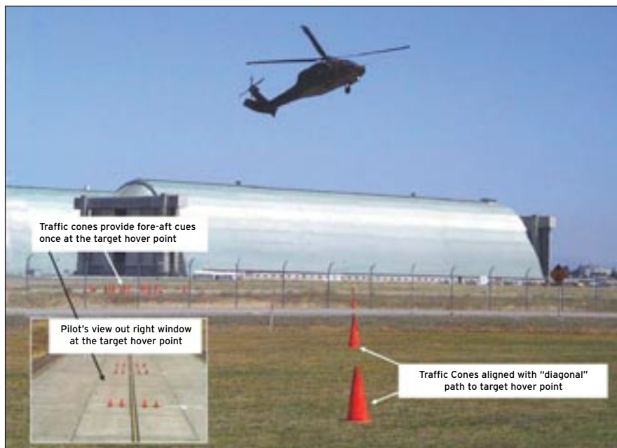
Hover MTE traffic cones course layout for UH-60A Black Hawk testing.
