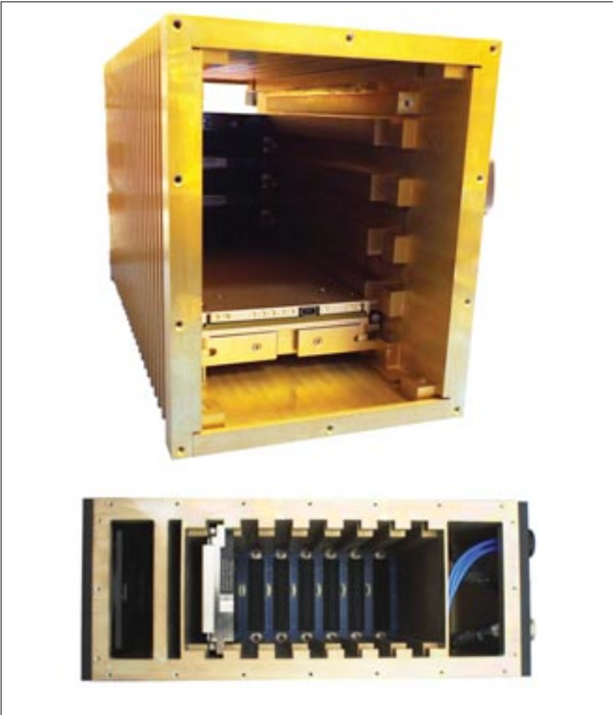
Figures 4a & 4b. For medium to high slot counts, a top-loaded approach for OpenVPX boards is common, as shown in Figure 4b (bottom). For smaller slot counts, a rear-loaded configuration, as shown in Figure 4a (top), allows a compact size in a rugged and secure I/O format.
