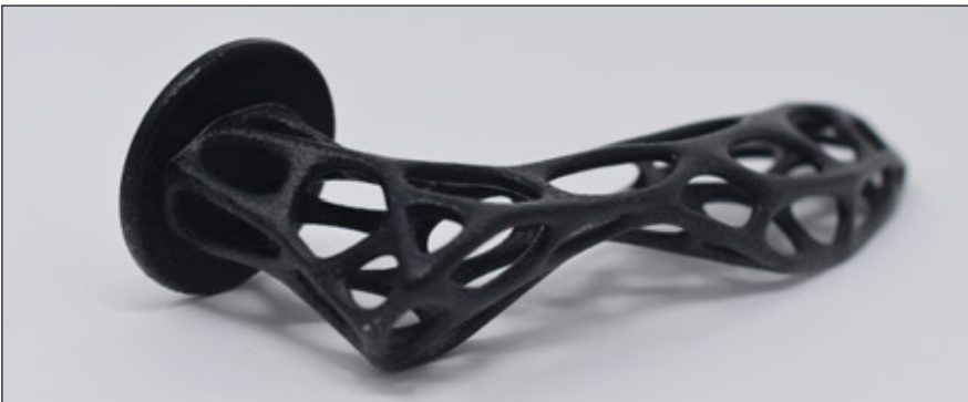
The PostPro3D BLAST process can achieve consistent surface finish on non-line of sight organic lattice structures.
