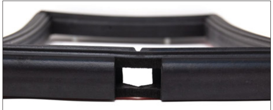
Water jet cutting can create precise holes, notches, and chamfers to accommodate fastener heads and enclosure features.
