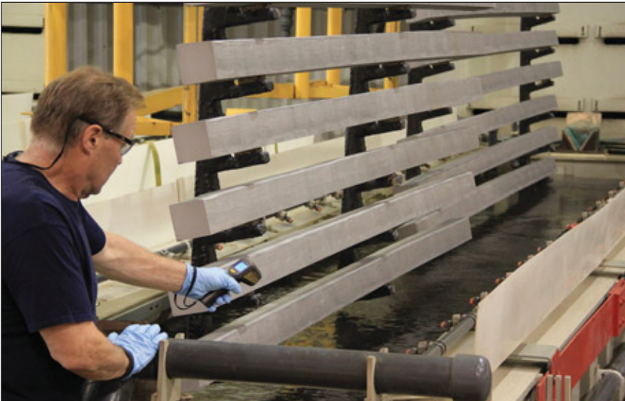
Technician checks electrochemical bath temperature as material is loaded into tank. The green MetCon process environment requires none of the extreme hazmat precautions typically associated with pickling.
