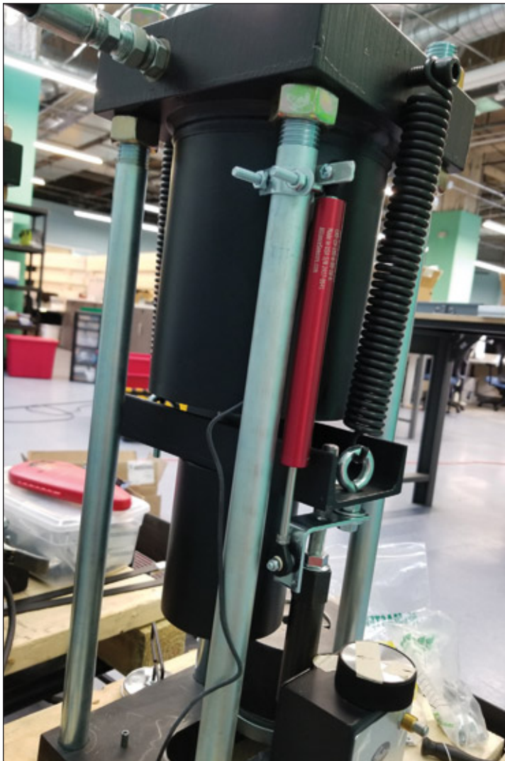
Figure 2. An LR-19 series LVIT (Linear Variable Inductance Transducer) position sensor installed on a crimping machine.
