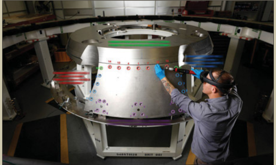
A Lockheed Martin technician using AR manufacturing instructions created with Scope AR's WorkLink platform. (Image credit: Lockheed Martin)
