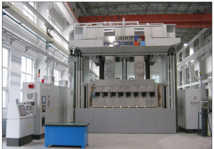
This 1200-ton SPF press manufactures aircraft panels for the Chinese aerospace sector.
