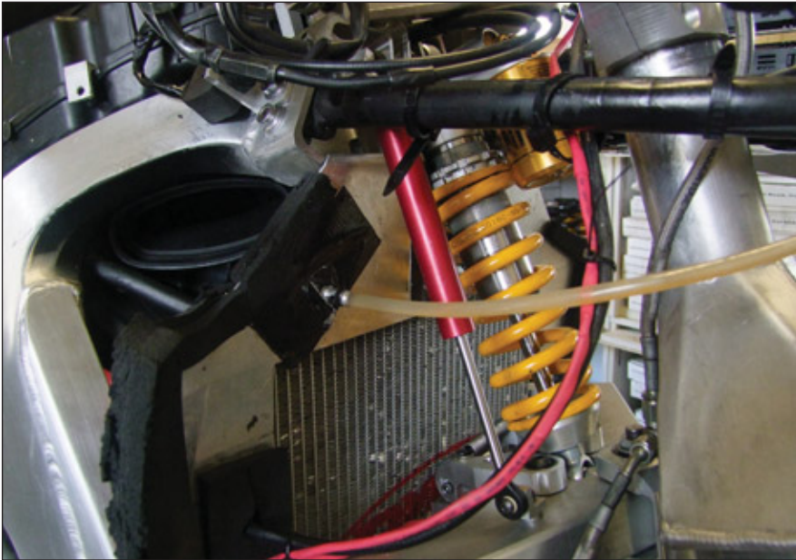
Figure 3. An LR-19 series LVIT (Linear Variable Inductance Transducer) position sensor installed in a vehicle suspension system.
