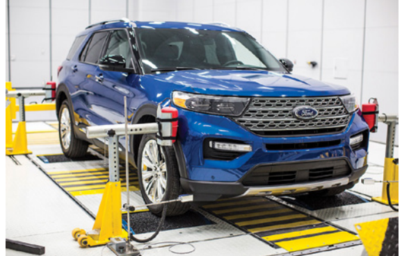
Ford’s new driving dynamics NVH lab includes a semi-anechoic chamber for full-vehicle validation testing.
