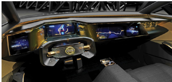
Although billed as a sport sedan, the IMs steering wheel retracts for SAE Level 5 autonomy if desired.
