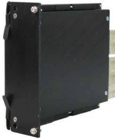
Figure 1. CompactPCI Serial has long been ruggedized for extreme environments. This SBC (courtesy of MEN Micro) shows an example of a 3U version in a conduction-cooled clamshell.
