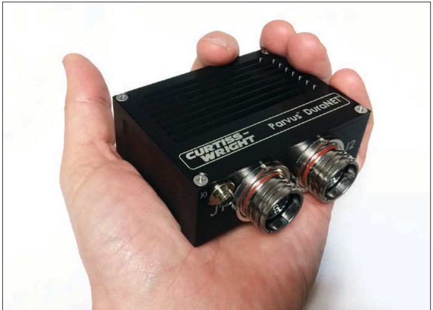
The Parvus DuraNET 20-11 is an ultra-small form factor (SFF) rugged Commercial Off the Shelf (COTS) 8-port Gigabit Ethernet (GbE) switch optimized for extremely demanding size, weight and power (SWaP) constrained vehicle and aircraft platforms exposed to harsh environmental and noisy electrical conditions (e.g. high altitude, extreme shock and vibration, extended temperatures, humidity, dust and water exposure, noisy EMI, and/or dirty power).
