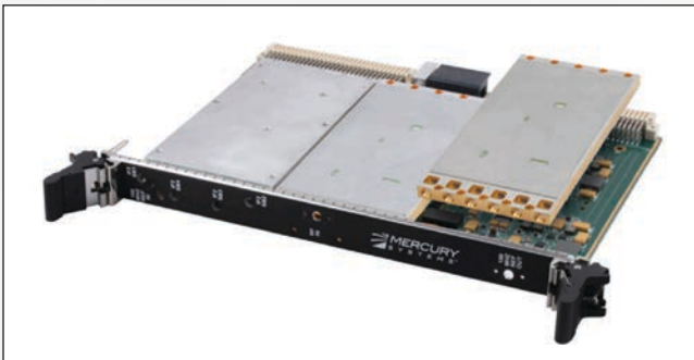
Figure 1. This is an OpenRFM module riding atop an OpenVPX board. Traditionally, the functions performed in the OpenRFM module would have been implemented in a larger separate housing.
