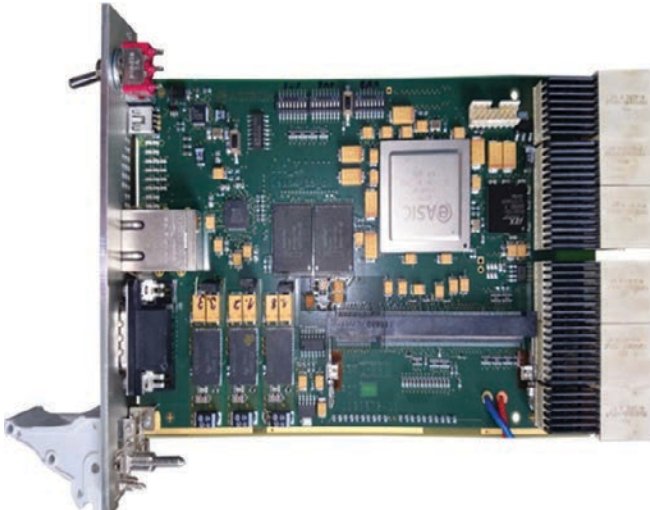
Figure 2. There are a variety of advanced processors being developed in CompactPCI Serial/cPCI Serial Space, including this SPARC-based Leon4 quad core board (right) and P4080 board (left). SPARC/Leon is a preferred platform computer used by the European Space Agency.
