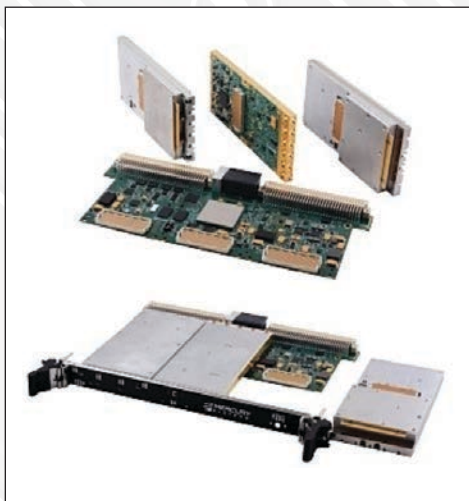
Figure 2. The 6U VME carrier (bottom) and three OpenRFM modules (top): a quad downconverter (left), wideband tuner (center), and direct-digital synthesizer (right).
