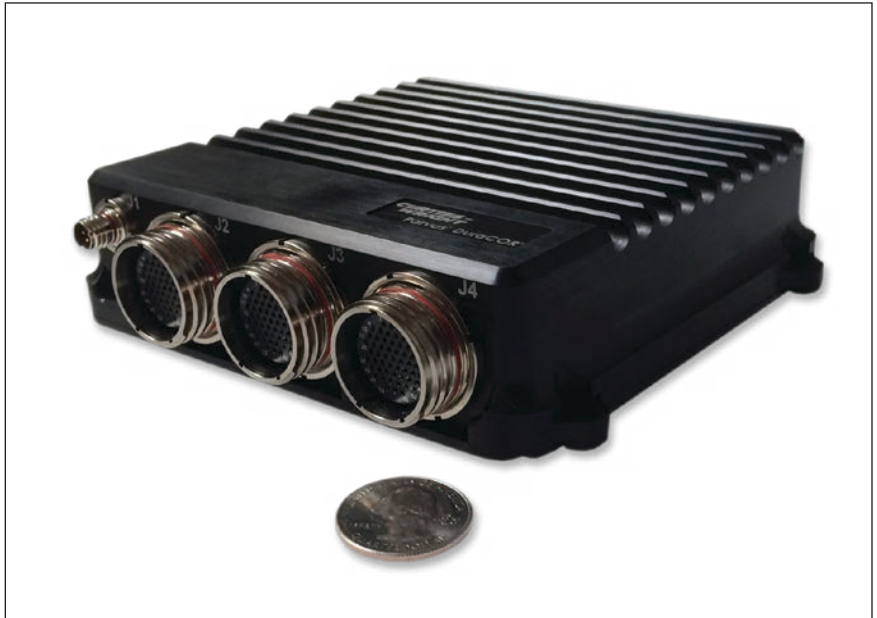
The Parvus DuraCOR 311 is an ultra-small form factor (USFF) rugged embedded computer/controller based on a low-power, quad-core Intel Atom 3845 (Bay Trail-I) processor equipped with a rugged flash disk and PCIe-Mini Card I/O expansion slots. Featuring a fanless IP67 design with MIL-performance connectors and extended temperature operation (-40 to +71°C), this miniature multi-core rugged Commercial Off the Shelf (COTS) processor is an ideal x86 mission computing solution for size, weight, power and cost (SWaP-C) sensitive applications.
