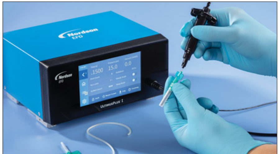
Dispensing UV-cure adhesive onto a kyphoplasty catheter. (Credit: Nordson EFD)
