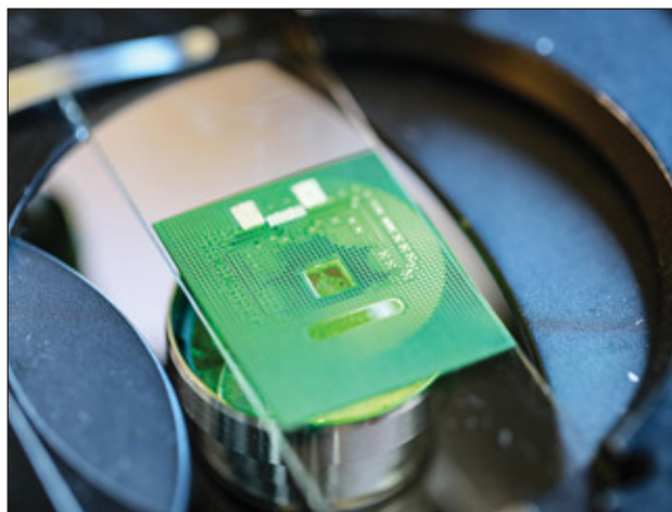
A microfluidic path brings the biofluids toward the chip. (Credit: EPFL)
