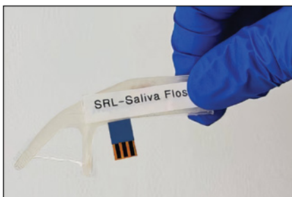
This dental floss pick has a sensor that can assess a person's stress level. (Credit: Atul Sharma and Nafize Ishtiaque Hossain)
