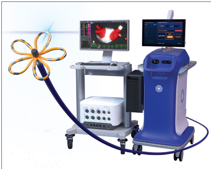
The FARAVIEW™ Software Module, coupled with the FARAWAVE NAV Pulsed Field Ablation (PFA) Catheter, provides an integrated solution for cardiac mapping and ablation procedures, specifically for treatment of atrial fibrillation (AFib). [Image provided courtesy of Boston Scientific. ©2025 Boston Scientific Corporation or its affiliates. All rights reserved.]
